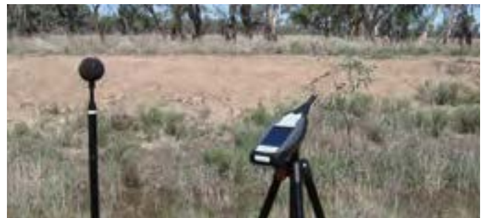
Sound monitoring equipment used for noise modelling.
